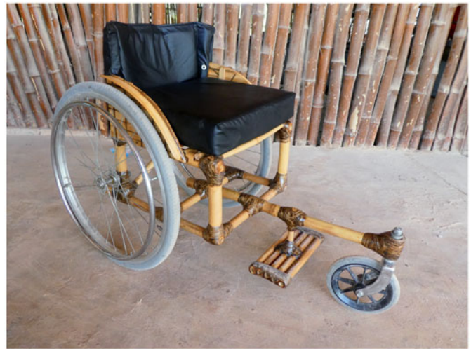
Figure 3. Rural wheelchair prototype design aiming to support wheelchair users in low-resource and tropical settings. Image © Marjelle F Scheffers.
