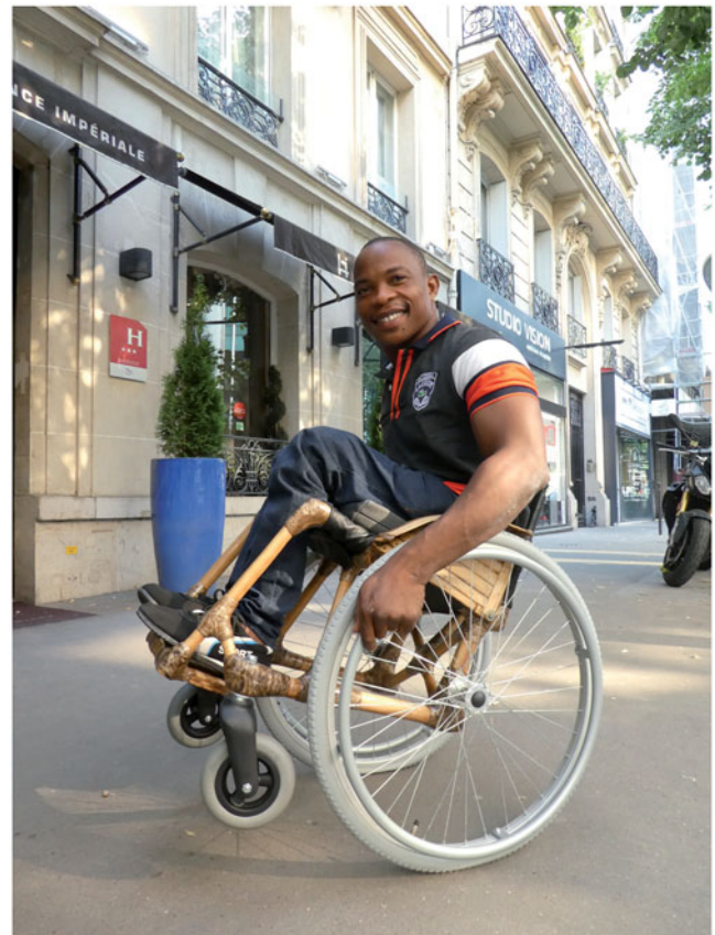
Figure 4. Urban wheelchair prototype design in use for testing and aiming to support wheelchair users in low-resource and tropical settings. Image © Marjelle F Scheffers.
