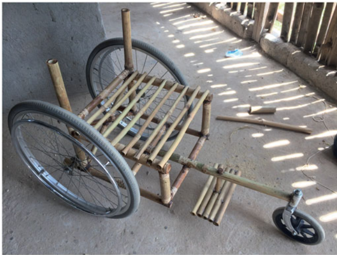
Figure 2. The skeleton of the rural wheelchair constructed with Bambusa vulgaris bamboo, Epoxy Steel ® and a conventional hot glue gun. Image © Marjelle F Scheffers.
